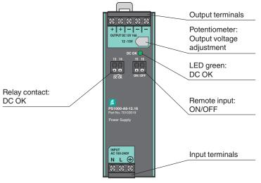
Mount the device on the DIN mounting rail so that the input terminals are located on the bottom of the device.
